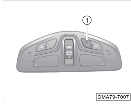
Emergency contact button
