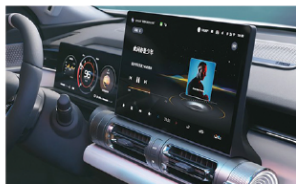
7" LCD Instrument Cluster & 10.1" Touchscreen with Wireless Apple CarPlay/Android Mirroring
